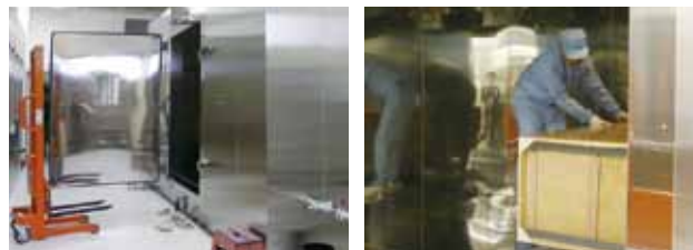
Using the large chamber to measure the emission rates of volatile organic compounds
